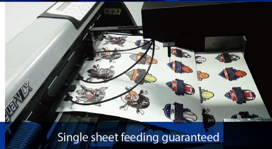
Suction cap for automated sheets feeding process
